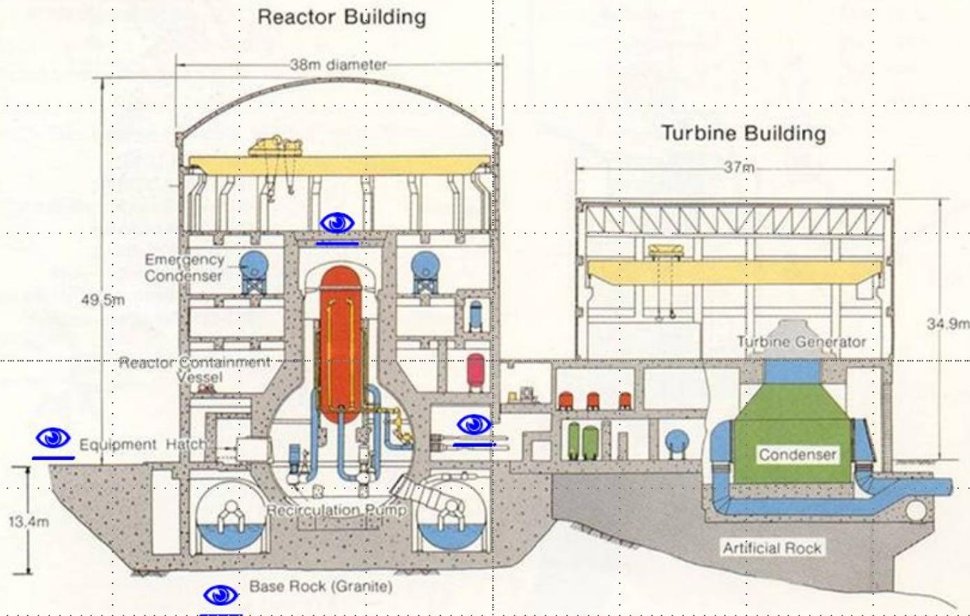
**The Mark I primary containment features a drywell (the inverted lightbulb) and a torus (the donut) connected by eight vent pipes. The reactor building surrounds the primary containment. Steam and feedwater piping passes through the containment walls and reactor building to the turbine building.**
